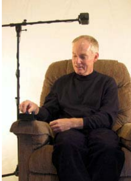
Fig. 1 – The receiver and loudspeaker of the SSSL, as set up for use.
